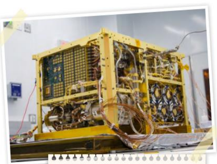
The Sample Analysis at Mars (SAM) instrument is a science laboratory on the Curiosity rover. This is a picture from before it was installed.
